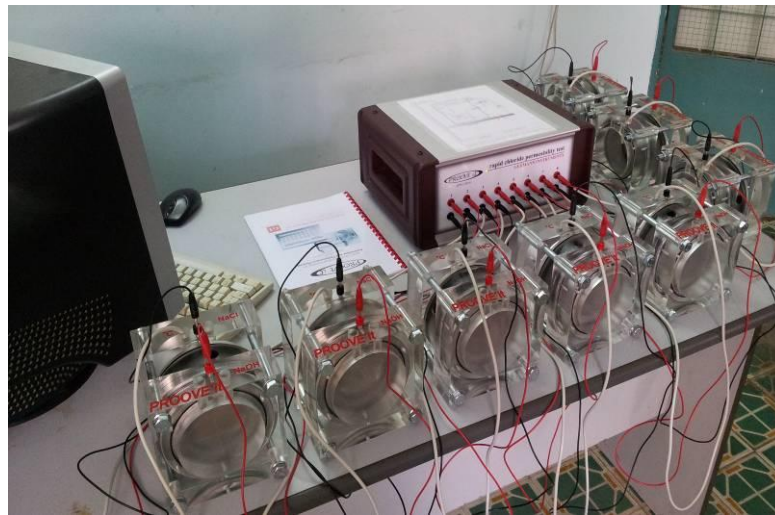
Figure 3. The automatic data processing equipment used to test the charge passed
