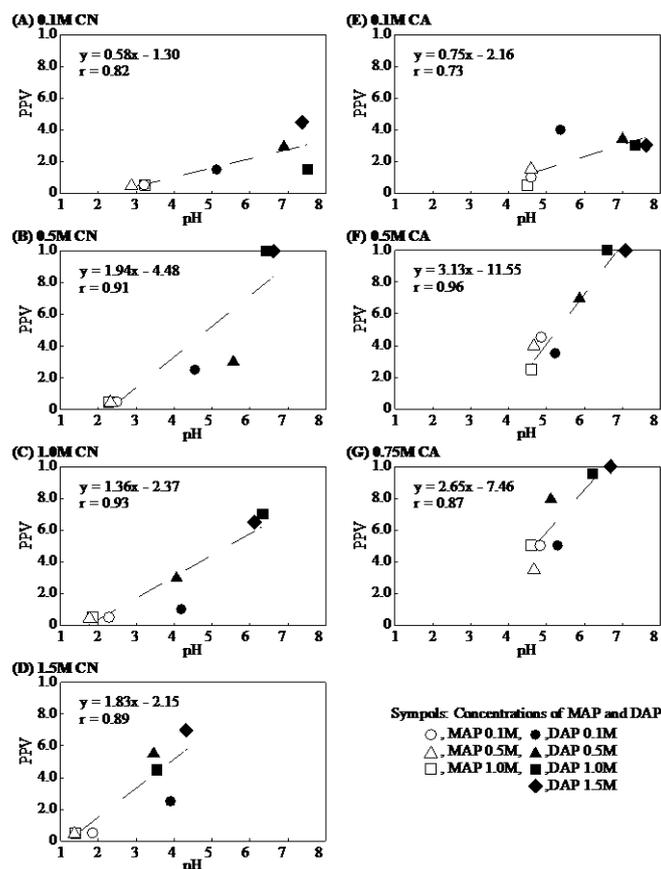
Figure 2. Relationship between the proportion of CPC precipitation volume of reaction mixture (PPV) and pH for calcium nitrate (CN) and calcium acetate (CA)
