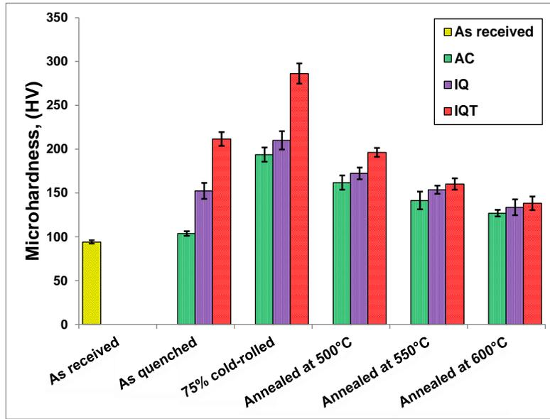
Figure 1. The microhardness values of specimen in various stage processes.
